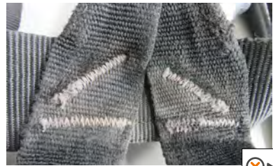
• Damaged safety stitching
