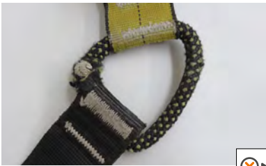
• Damaged attachment point
